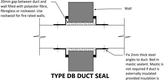
(Note: Typical fire damper detail is also adequate provided flange is sealed to wall with Selley's Fire Block)
