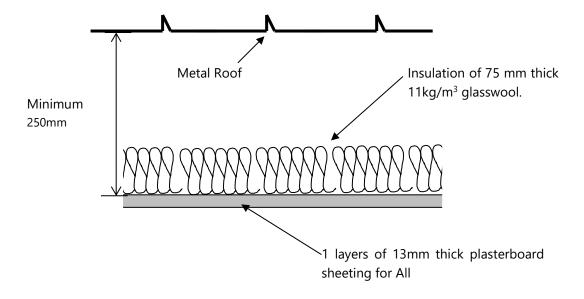
Penetrations in ceilings (such as for light fittings etc.) must be sealed gap free with a flexible sealant. Any ventilation openings in the ceilings would need to be acoustically treated to maintain the acoustic performance of the ceiling construction.
